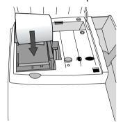
3. Feed the free end of paper through the gap in the cover.
