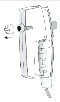
When the hand unit is removed from the holster the two green LED's on the front illuminate, and the pump starts (an audible tone is emitted). The pump takes 2 seconds to prime before the unit is operational.
